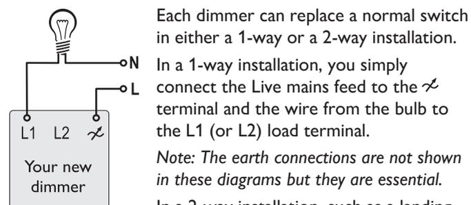
In a 2-way installation, such as a landing light that can be switched from downstairs as well as upstairs, the wiring will be achieved in either of two ways:
